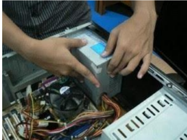
Gambar 2.13 memasang power supply
