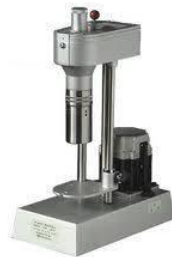
Gambar 2.2 Viskometer Cup and Bob
